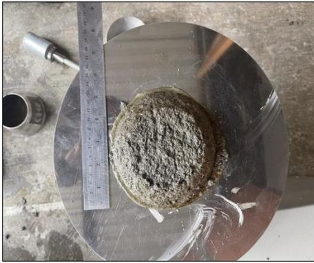
Gambar 6. Uji Sebar Mortar Normal
