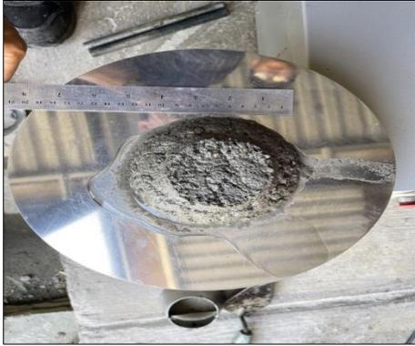
Gambar 7. Uji Sebar Mortar Papercrete
